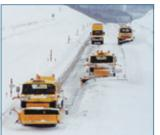
A group of three snowplows and a VMS vehicle is working together to clear entire lanes. So long as this work is going on, passing is not possible.
