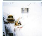
Snow pushed onto the shoulders of roads is cast off the road by rotary-type snowplows.
